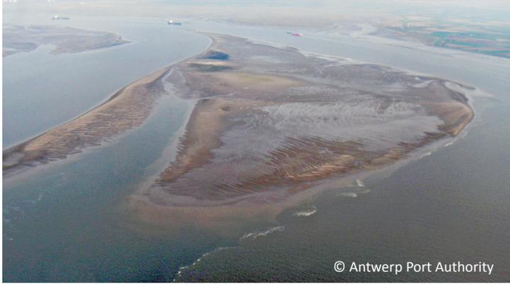
Since 2001, this new disposal strategy has been investigated as a pilot project on the sandbar at Walsoorden. Extended research was conducted to evaluate the feasibility of the site and two disposal tests were carried out (2004 and 2006). The tests were monitored thoroughly from 2004 up to 2009, and results showed a successful outcome: the disposed material seemed to remain in place, and from an ecological viewpoint no negative effects were observed.
