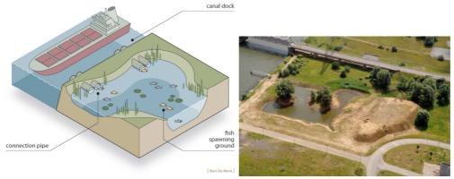
Figure 3. Left: Scheme of a fish spawning pond (Bart De Neve); Right: a picture of the Antwerp fish spawning pond
