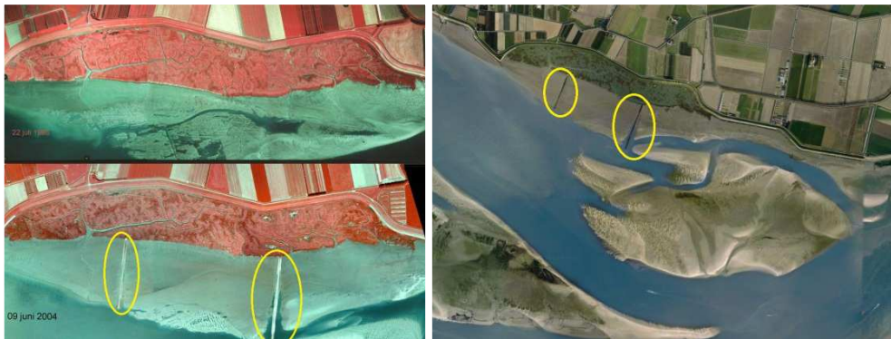
Figure 2. LEFT: Situation 1998 and 2004 (1 year after completion). Situation 1998 (up) shows the remains of the flooded 17th century village. Situation 2004 (down) shows the groynes and the sedimentation that already took place after one year. RIGHT: Air view of the study area (after completion)
