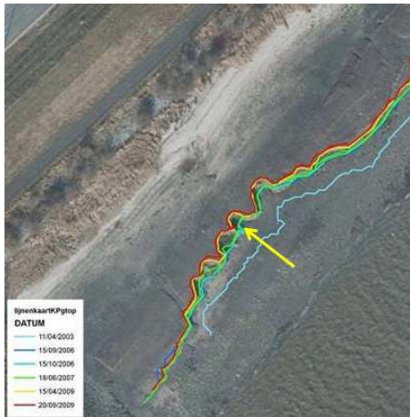
Figure 6. Evolution of the top of the cliff at zone G, 2003-2009 (Speybroeck et al. 2011).
